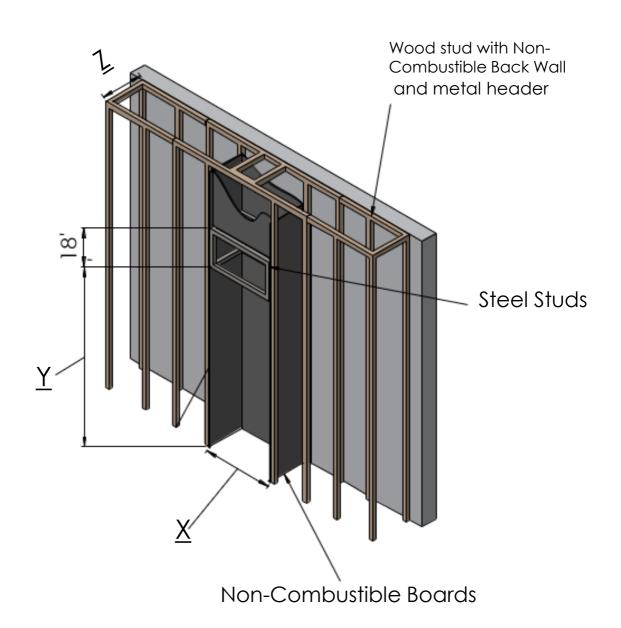
NOTE: Dimension 'Y' uses legs at default lowest height 4" below the unit with glass beginning 10" above the floor. Increase leg height and Y dimension for higher viewing window.
