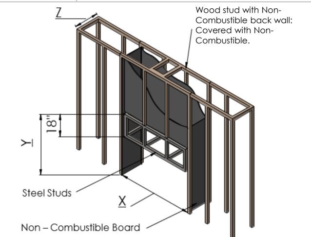
NOTE: Dimension 'Y' uses legs at default lowest height 4" below the unit with glass beginning 10" above the floor. Increase leg height and Y dimension for higher viewing window.
