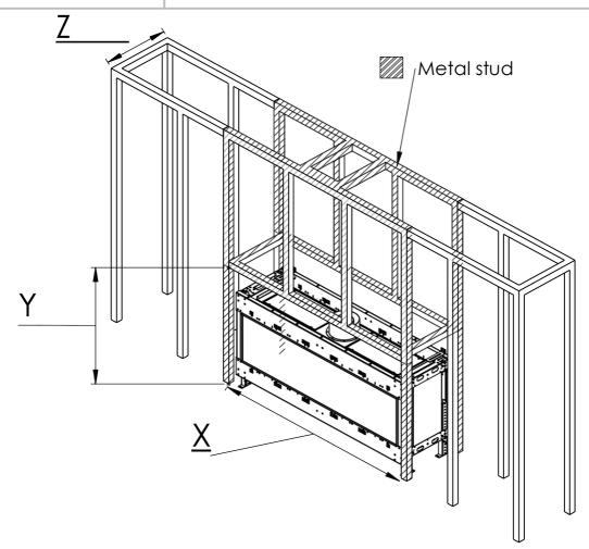
**NOTE**: Dimension 'Y' uses legs at default lowest height 4" below the unit with glass beginning 10" above the floor. Increase leg height and Y dimension for higher viewing window. All framing and finishing must be secured to your projects back wall, ceiling or floor, and must never bear weight on the fireplace in any circumstance. For more information reference the <u>Installation Manual</u>
