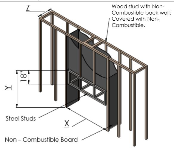
**NOTE**: Dimension 'Y' uses legs at default lowest height 4" below the unit with glass beginning 10" above the floor. Increase leg height and Y dimension for higher viewing window. All framing and finishing must be secured to your projects back wall, ceiling or floor, and must never bear weight on the fireplace in any circumstance. For more information reference the **Installation Manual**
