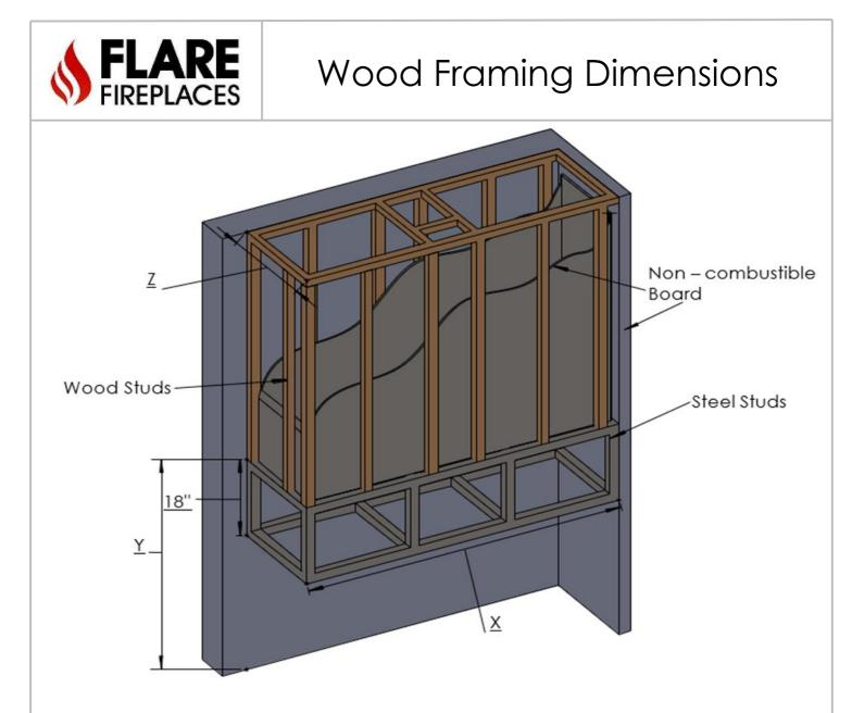
NOTE: Dimension 'Y' uses fireplace at default lowest height with glass viewing window beginning 8 ¼" above the floor. Any higher viewing windows must have a platform created to raise fireplace off the floor and Increase the value of 'Y' to accommodate any increase.
