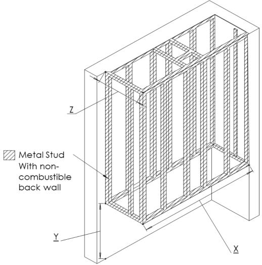
NOTE: Dimension 'Y' uses fireplace at default lowest height with glass viewing window beginning 10" above the floor. Any higher viewing windows must have a platform created to raise fireplace off the floor and Increase the value of 'Y' to accommodate any increase.
