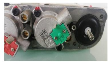
6) Using a suitable screwdriver tighten the marked screws as shown in the image below:
