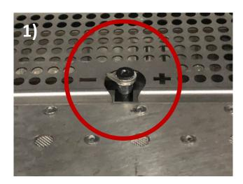
2) Using a phillips head screwdriver adjust mix of air & gas needed for a natural looking burn. See images below for what each setting achieves.
