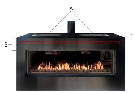
NOTE: If choosing to place the heat release on the face of your surround, instead of centered on top of the surround, the opening must be on both the front and back of the cavity. It cannot only be on the short-sides but can be on all sides.
