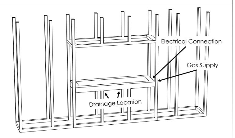
**Drainage**- Flare Fireplaces Vent Free line are outdoor rated using Stainless Steel, corrosion resistant materials. However, care should be taken to ensure rain and other moisture cannot collect between unit and mounting platform. Plan for drainage to run outside of cavity away from other fixed buildings and objects.
